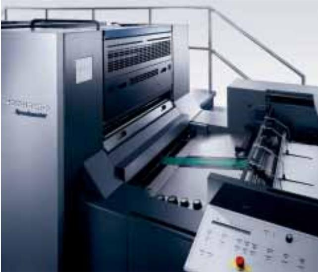
When changing format or printing stock, the feeder with central suction tape gets production off to a fast start.
